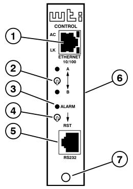
Figure 2.2: The Control Module
